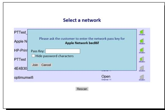
The ps-iLevel will now verify your password and join the network. The configuration settings will be saved to allow the iLevel to reconnect to the network automatically on powering up.
